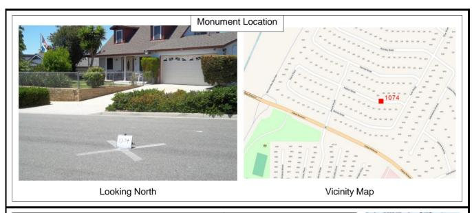
**Monument Description:** GPS Useable: Full stamping: USCE La-Dist SIr Yes 2010-22 By Johnson Frank Gear Spike in AC With Washer Stamping: SLR 2010-22 Center Mark: Depth: Punch 0 Recovery By: Lid: RBF Date: August 2013
