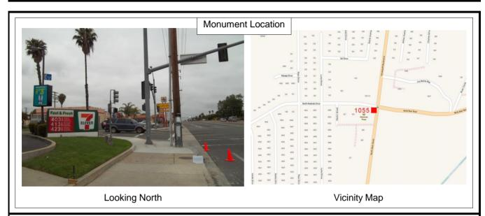
Monument Description: GPS Useable: Additional Stamping: City of Yes Oceanside Survey Control Station 2.5" Brass Disk set in Curb Inlet 1055 2013 Stamping: LS 7854 Depth: Center Mark: Triangle / Punch 0 Recovery By: Date: Lid: RBF June 2013
