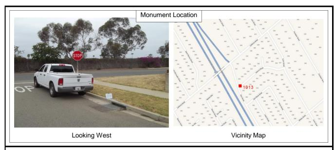
Monument Description: GPS Useable: Additional Stamping: City of Yes Oceanside Survey Control Station 2.5" Brass Disk set in Curb 1013 2013 Stamping: LS 7854 Depth: Center Mark: Triangle / Punch 0
